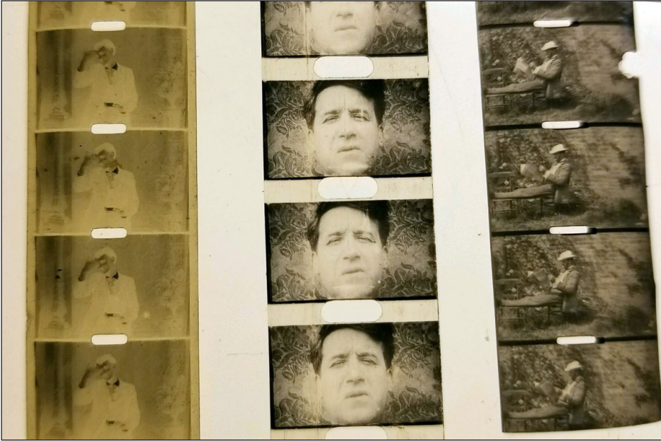
FIGURE 1. Examples of 17.5mm film from the USC Hugh M. Hefner Moving Image Archive. From left to right: Ernemann Kino (1903), Ikonograph (1907), and Biokam (1899). Photograph by Dino Everett, USC.
