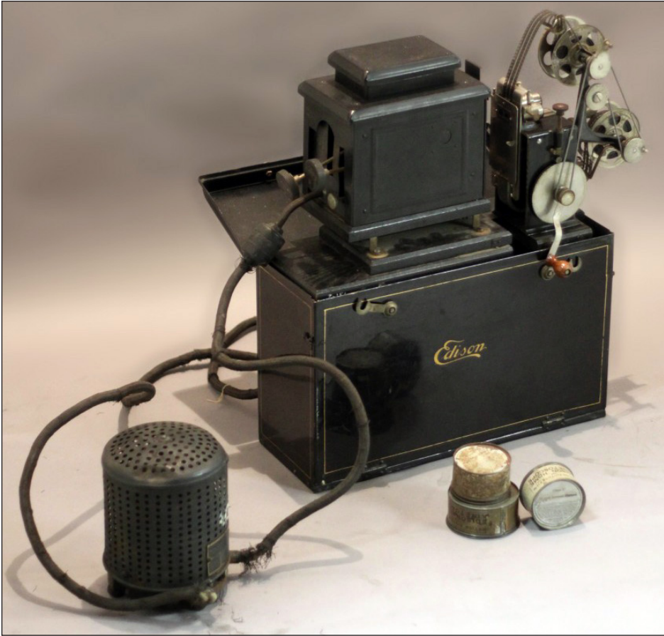
FIGURE 11. 22mm Edison Home Kinetoscope Projector. Photograph by Dino Everett, USC.
